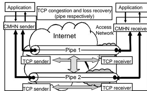
Figure 1: Architecture of the proposed scheme
