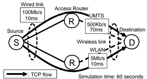
Figure 3: Simulation model
