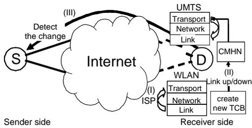
Figure 2: Detection procedure (WLAN link)
