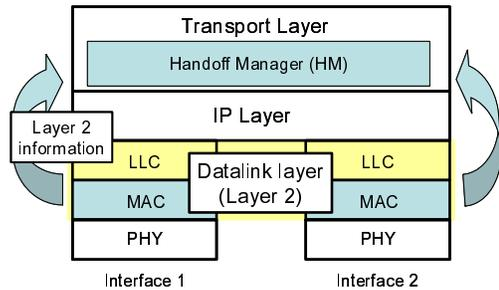
Fig. 1. Cross-layer architecture.
